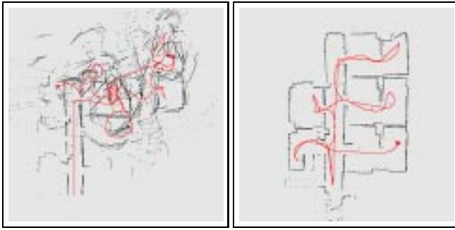
Figure 9: Autonomous exploration and mapping using the urban robot: Raw data and final map, generated in real-time during exploration.
